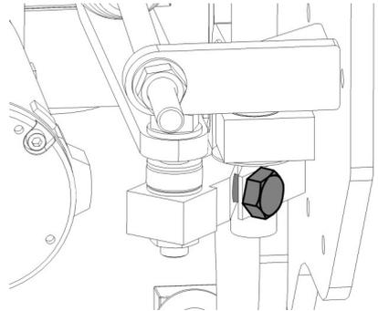
4. Rotate the rear pusher anti-clockwise (when viewed from above) until the nylon roller is just clear (2-3mm gap) inside the notch at the rear of the top plate.
