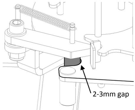
5. Tighten the rear pusher clamp block bolt
