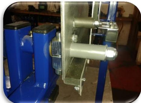
Ensure clamp block is in start position (pins touching).
