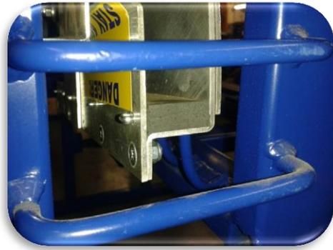
Tighten the Hex bolt to fix the throwing tray clamp block.
