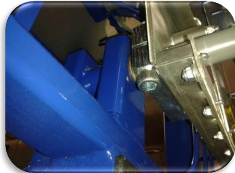
On the outside of the arm, there is a grey plastic tube with a Nyloc nut. Turn the Nyloc nut half a turn.
