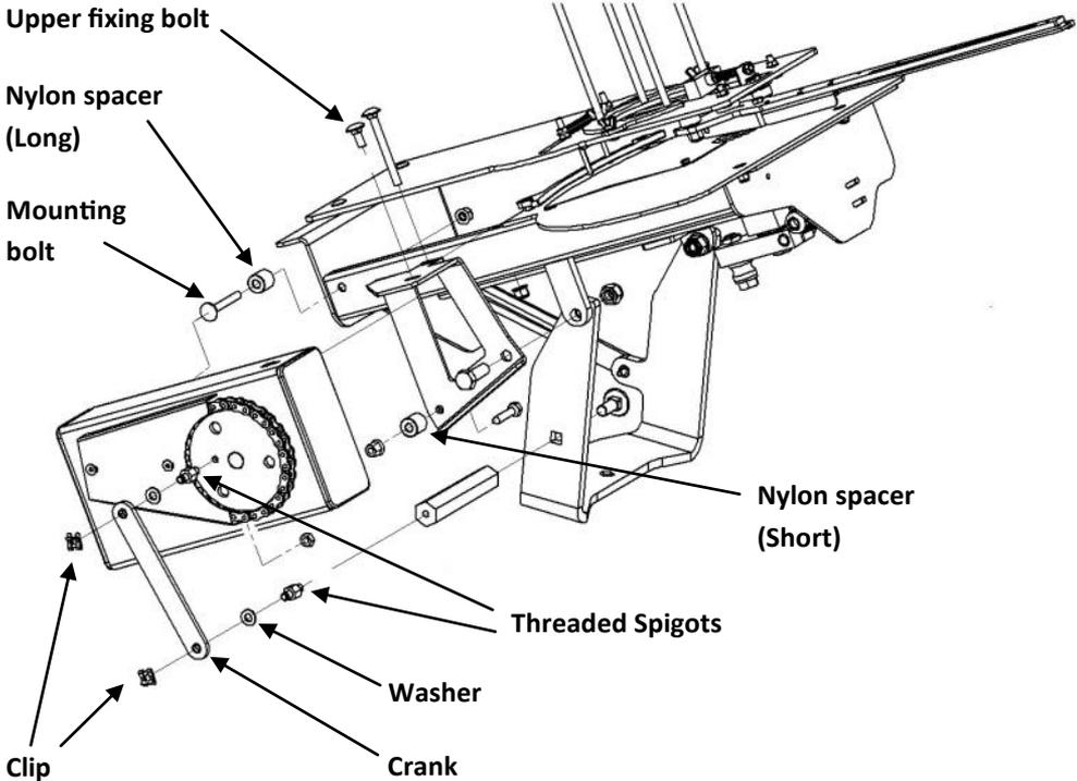
Each of the threaded spigots should now be fitted with a lightly greased washer, followed by the crank fitted between them. The crank is secured by a spring clip at each end which simply slides into the fine groove, snapping in place over the end of the shaft.
